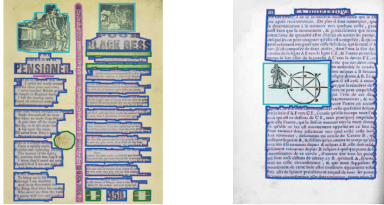
Figure 2. Sample images showing the region outlines (blue: text, magenta: separator, green: graphic, cyan: image).
