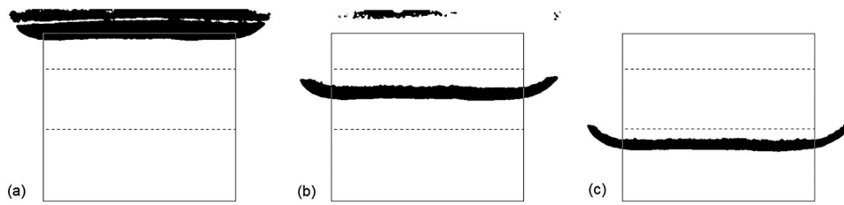
Figure 4. Binary (black and white) image analysis with the dewaterability estimation test software: (a) start of the test and waterfront development; (b) the waterfront has passed the first line of interest; (c) the waterfront has passed the second line of interest.
